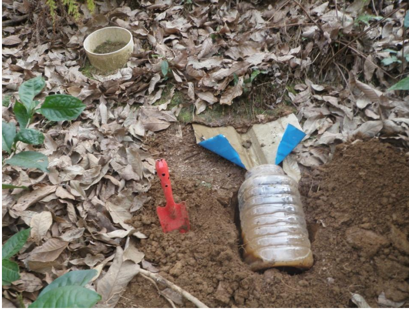
Figure 3. Diagram for collecting runoff water and drained soil. The blue steel frame inserted firmly in soil and the plastic jar is used for collecting water and soil. [I think we can improve on the design of this trap. The bottle needs to be bigger and connected to the sheet with a pipe. The bottle is dug into the soil 1-2 m below the trap to minimise disturbance. The sheet could also be better (flatter with edges down the sides)]
